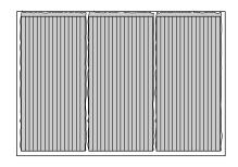
Figure 21 - Correct Burner Flame Pattern
